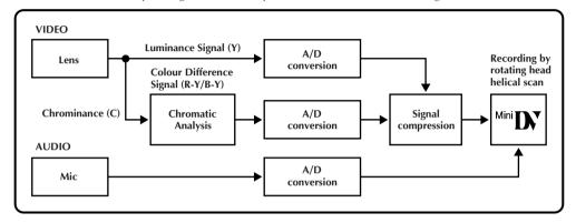
This camcorder separates the data into blocks, writing one block of each data type on each track of the tape.
